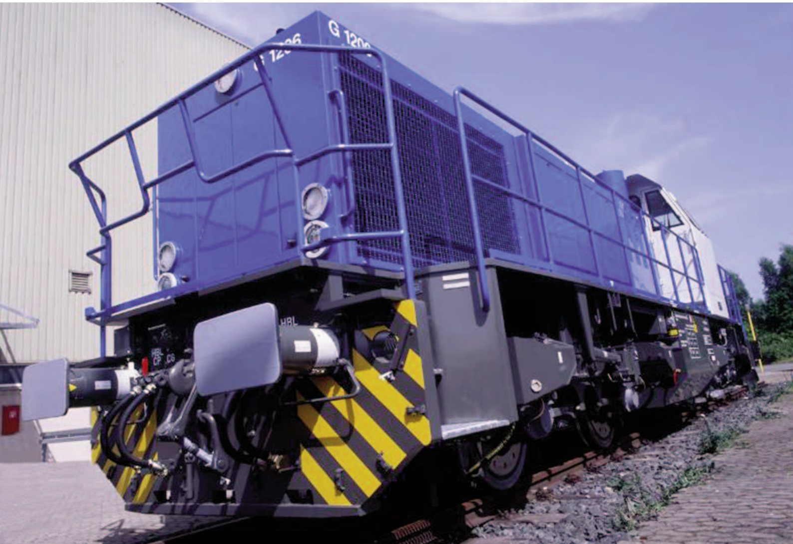
Diesel-hydraulic locomotive G1206
