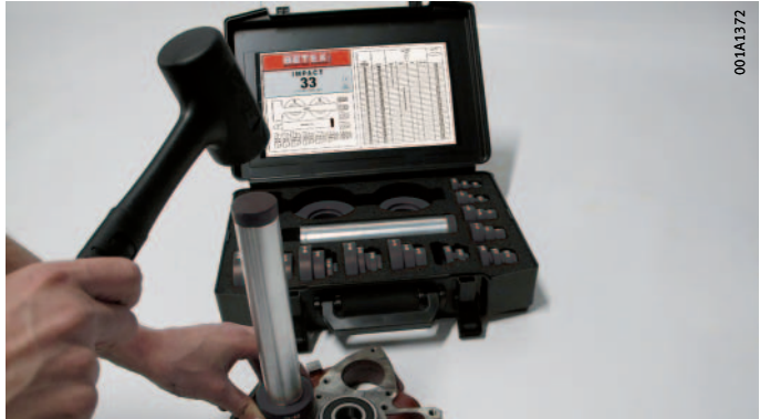
Figure 3 Bearing installation with hammer and mounting sleeve set
