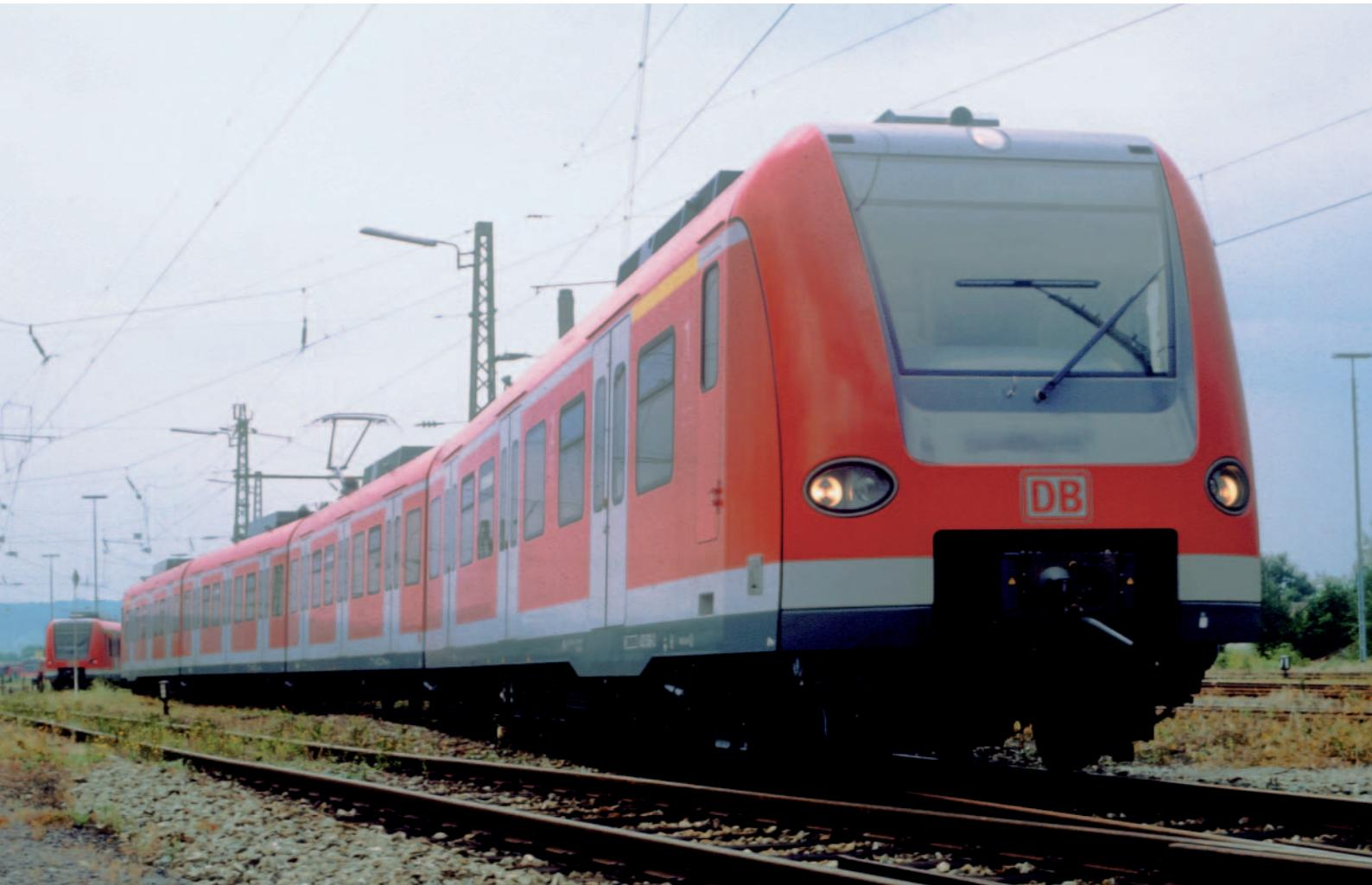
Class 423 electrical multiple unit: Developed by a consortium of Bombardier Transportation and Alstom LHB in cooperation with DB AG
