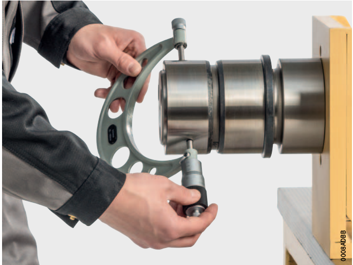
Figure 3 Measurement of expansion using external micrometer
