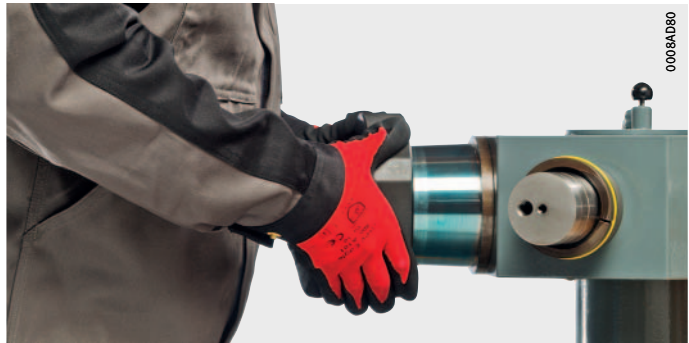
Figure 5 Touching with a taper ring gauge
