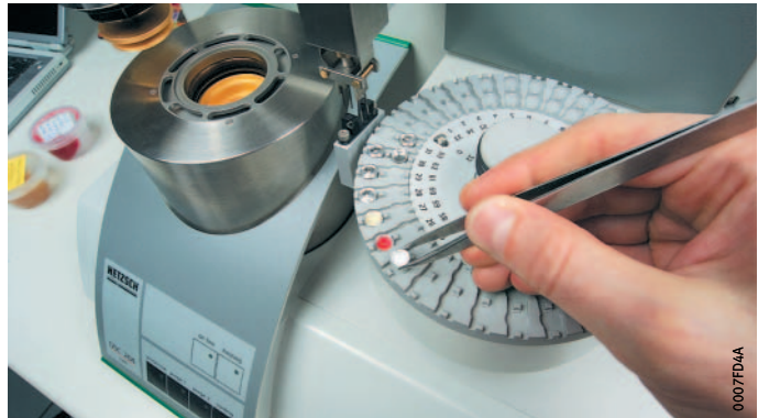
Figure 5 Analysis of the thermal behaviour of greases
