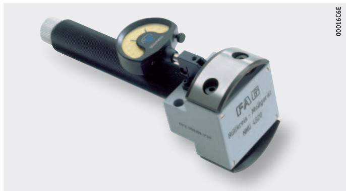
Figure 8 Enveloping circle gauge FAG MGI 21
