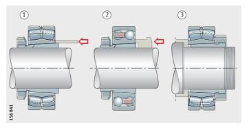
The dismounting of large bearings located using a withdrawal sleeve requires considerable force. In this case, locknuts with additional pressure screws can be used, *Figure 8*. A disc must be inserted between the inner ring and the pressure screws in order to prevent damage to the bearing.
