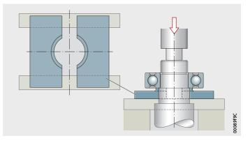
*Figure 3* Dismounting using a press
