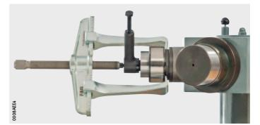
Figure 7 Two-arm extractor with hydraulic pressure tool
