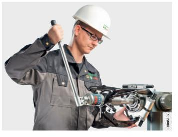
*Figure 1* Dismounting by means of extraction device
