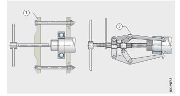
Extraction device with tie rods and split ring
