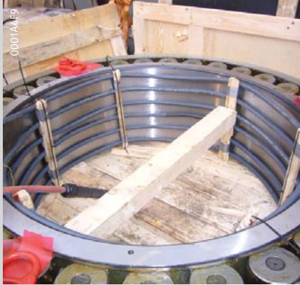
Heating of a spherical roller bearing
