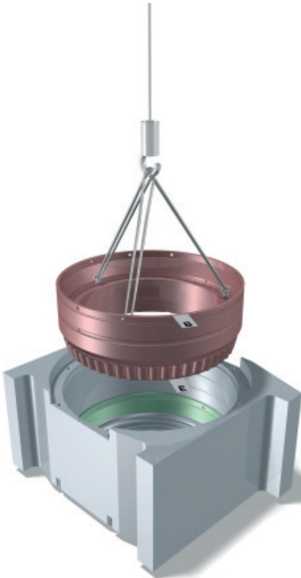
5: Mounting cone E-Ce, spacer C, cup B-D and spacer B (bearings with a pin-type cage)
