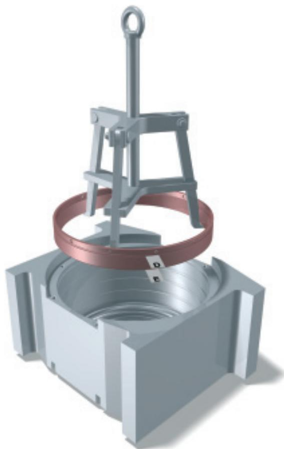
4: Mounting the cup D-E and spacer D
