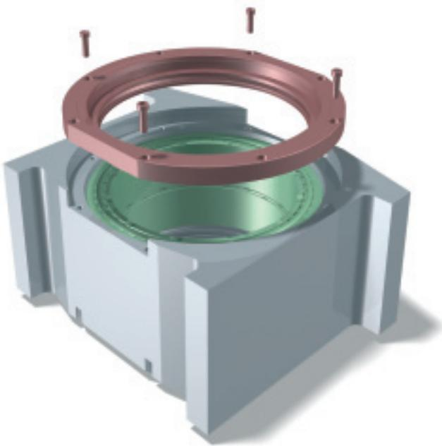
7: Mounting the chock cover without sealing ring
