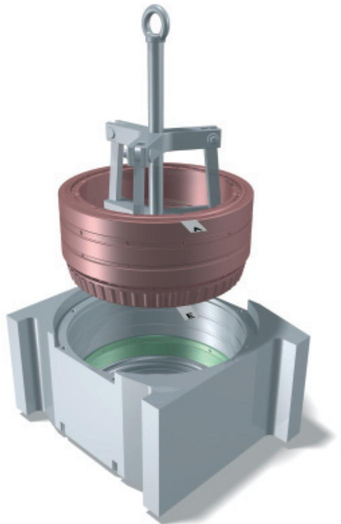
4a: Completing the bearing set (bearings with a pressed cage)
