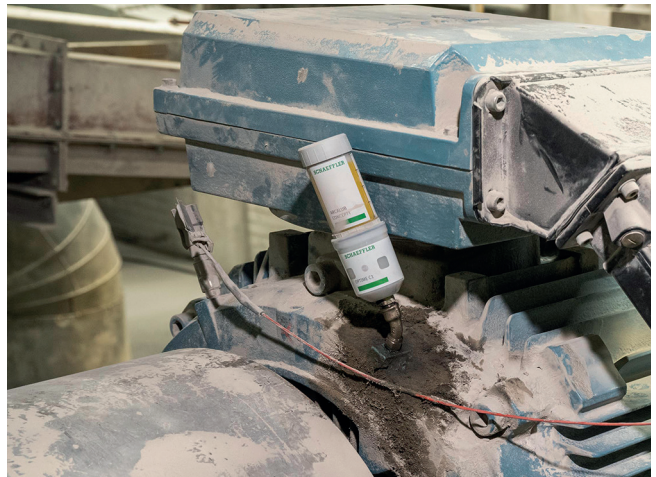
Lubrication solution Cement: OPTIME C1 lubricates with pinpoint accuracy and, thanks to smart technology, always indicates the status on a (mobile) end device regardless of location
