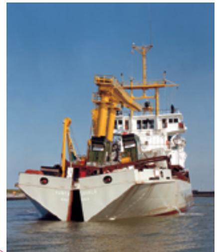
Special vessel for discharging gravel: Bottom washouts can be filled economically
