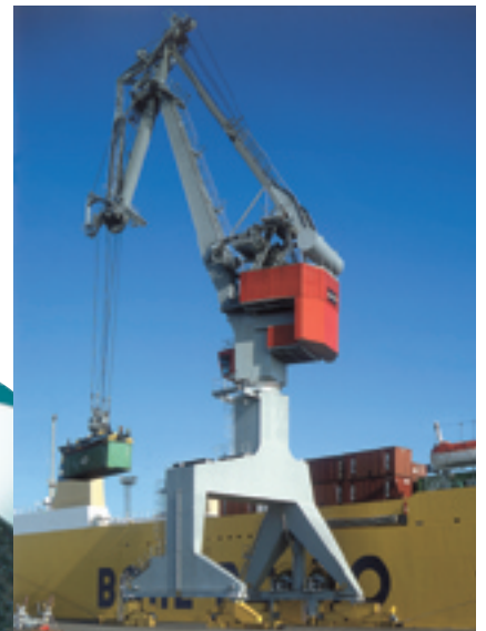
Slewing portal crane with double-link boom system: Tightly sealed ELGES bearings withstand aggressive environmental forces
