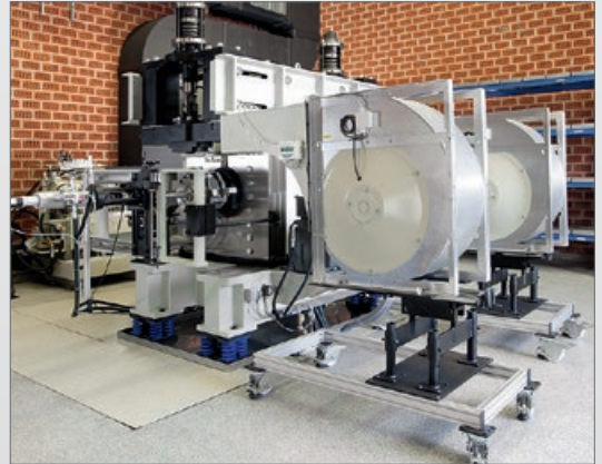
Railway applications – axlebox bearings EN12082 performance testing
