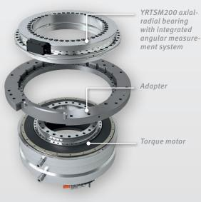
The idea is both simple and ingenious: Torque motor and rolling bearing are joined by ring-shaped adapters to form a ready-to-operate and perfectly matched unit. An angular measurement system that is integrated into the bearing can also optionally be included in the scope of delivery. Motor, adapter, and bearing (with or without the angular measurement system) are assembled by Schaeffler and delivered as a unit.
