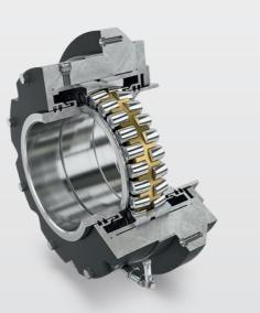
FKC flanged housing units comprise a housing body that is also available in current-insulated form where necessary, two labyrinth covers, two labyrinth rings, and two sealing sleeves that are used to support an additional sealing cover.
