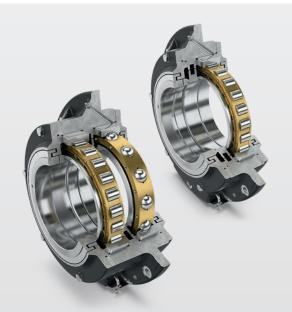
FERS and FERB series flanged housing units are designed according to the modular concept, i. e. the labyrinth ring, cover, spacer ring, grease valve, and the shaft nuts for locating the bearings are matched to each other.
