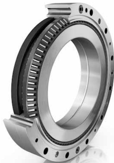
Schaeffler has developed a completely new bearing type specially for the articulated arms of lightweight robots and cobots: The double-row XZU-series angular contact needle roller bearing. The new series was optimized for outstanding tilting rigidity and reduced, uniform frictional resistance. One of the special features: The angular contact needle roller bearings have the same cross-section as the crossed roller bearings that are frequently
