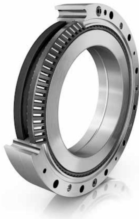
Schaeffler has developed a completely new bearing type specially for the articulated arms of lightweight robots and cobots: The double-row XZU-series angular contact needle roller bearing. The new series was optimized for outstanding tilting rigidity and reduced, uniform frictional resistance. One of the special features: The angular contact needle roller bearings have the same cross-section as the crossed roller bearings that are frequently
