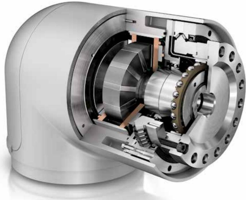
Schaeffler's new frameless UPRS-series motors offer a smaller design envelope, reduced weight, a higher torque density, and increased dynamics. These motors are designed as axial flux motors. The conventional coils in PCB design (printed circuit board) enable a very high torque density and excellent heat dissipation to the outside. The weight of the active components was reduced through the use of innovative materials. The reduced weight and improved performance data of the motors
