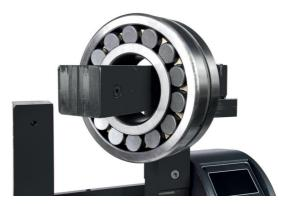
Always make sure that the workpiece does not come into contact with the plastic casing of the heater. When the heating is finished, follow the instructions in reverse order. Use heat-resistant gloves to move the heated workpiece.
