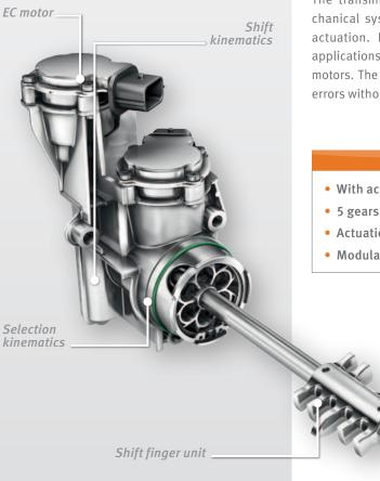
The transmission actuator is a modular electromechanical system that works independently of clutch actuation. It operates transmissions for AMT/DCT applications using two efficient, brushless electric motors. The active interlock principle prevents shifting errors without the need for additional sensors.
