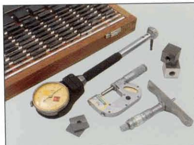
GAGES AND GAGE BLOCKS Accurate to .0001".
