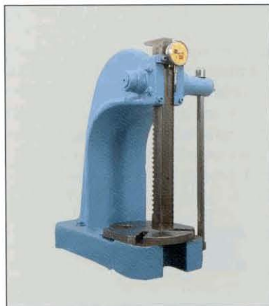
An arbor press is used for interference fits with small shaft/small bore instrument bearings.
