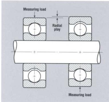
Radial internal clearance is measured under a light reversing radial load and corrected to zero load, to establish radial play values.
