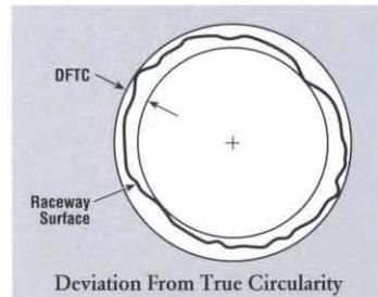
DFTC (deviation from true circularity) measurements are made and graphically depicted by concentric circles enclosing the low and high points of raceway deviation.
