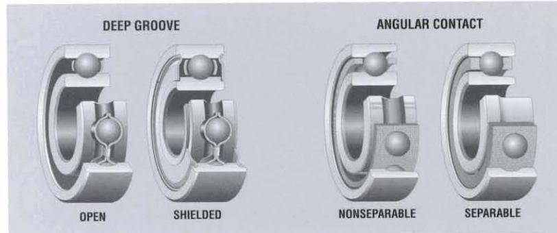
Design selections between deep groove and angular contact precision bearings depend primarily upon application characteristics such as magnitude and direction of loading, operating speed and conditions, lubrication, and requirements for accuracy and rigidity.
