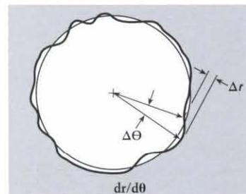
$dr/d\theta$ . (change in radius with a change in circumferential location) measurements are made to define lobing or waviness that could generate noise and vibration in an operating bearing.
