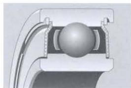
**Flexeal™** is a Barden-developed seal with a layer of fiber bonded to a precision aluminum stamping. The fiber is prelubricated to produce extremely low friction at the ground sealing notch. This low friction allows Flexeal equipped bearings to operate at speeds up to 600,000 dN. Maximum temperature is 300°F continuously, 350°F intermittently.
