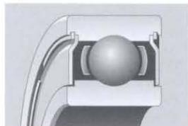
**Shields** are precision-stamped of stainless steel in a dished shape to provide rigidity, resistance to resonant vibration and maximum lubricant space within the bearing. Inner ring notches are provided where space permits, to present a difficult entry path for contaminants.
