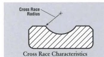
**Cross race characteristics.** Radius form, waviness and surface finish are closely monitored by Barden, using laser and computer technology. With equipment unique in the industry, cross race traces are made for comparison with Barden standards.
