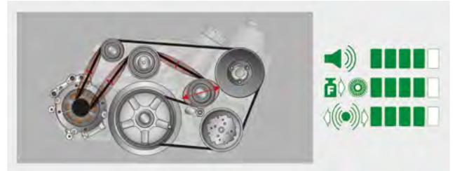
Since the multi-ribbed belt is vibrating, all components in the front end auxiliary drive are subject to stronger forces, resulting in greater wear. The associated damage can ultimately lead to overall system failure.
