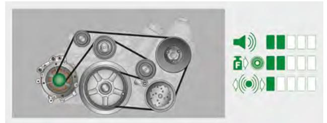
An INA OAP minimizes vibration of the multi-ribbed belt and thus protects all components in the front end auxiliary drive – doubling their service life.
