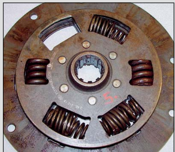
Torsion damper contaminated with oil/grease
