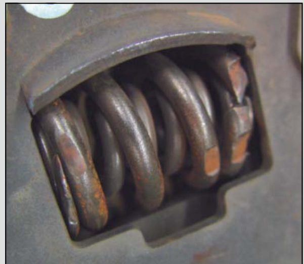
Torsion damper wear and fractures
