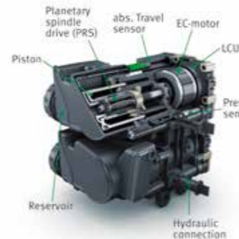
図3 HCA (Hydrostatic Clutch Actuator)
