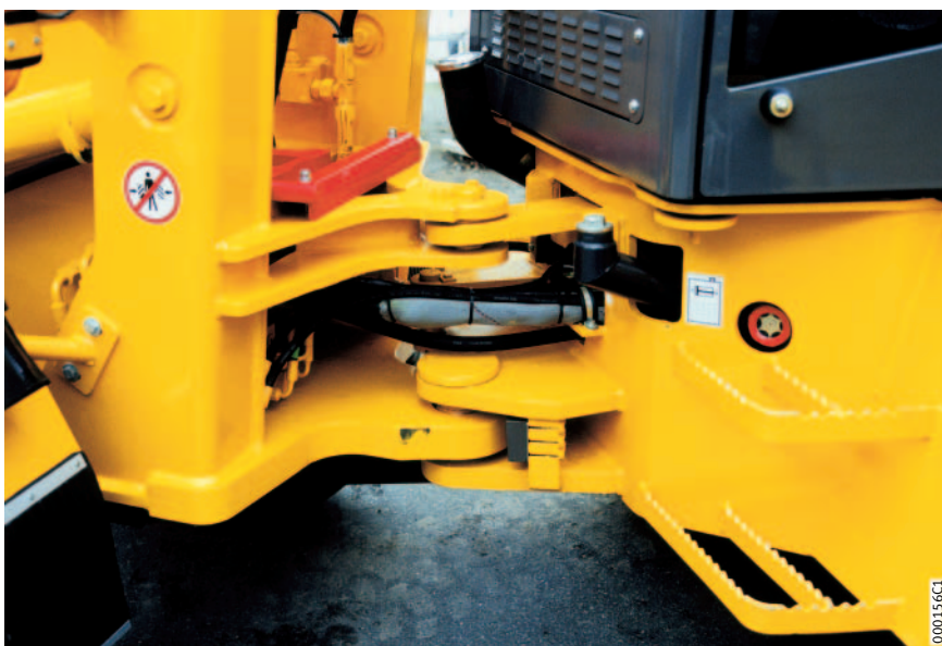
Figure 3: Articulation/swivel joint with ELGES spherical plain bearings
