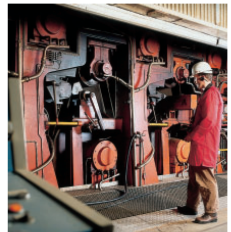
Condition monitoring of rolling bearings with the FAG Bearing Analyser
