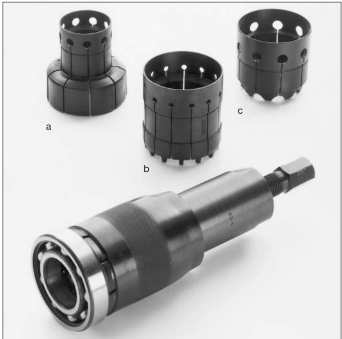
89a: Collet for tapered roller bearings and cylindrical roller bearings with separable outer rings/cups
