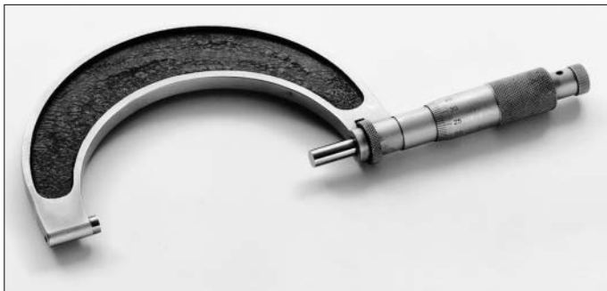
2: External micrometer for measuring shaft diameters
