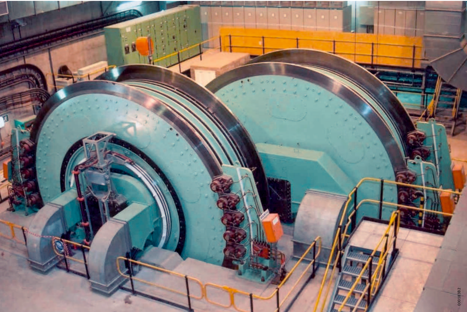
Figure 1 - Winder from SIEMAG TECBERG, Palabora Mining Company, South Africa
