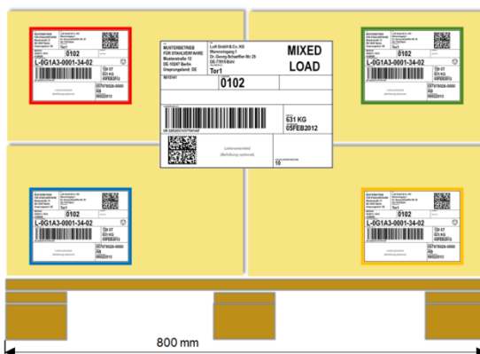
Fig.3 Example for the use of the MIXED LOAD label on a non homogeneous pallet (1200x800)
