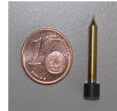
Minimized punch (weight: 0,8 g)
