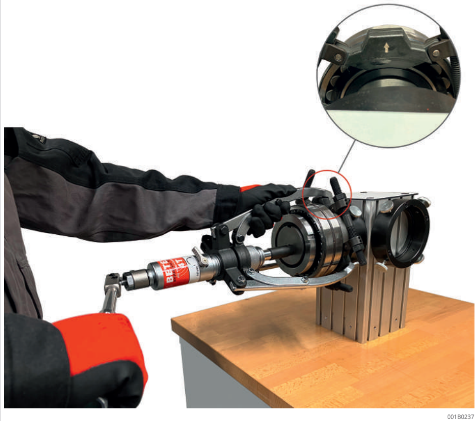
28 Dismounting with the TRI-SECTION-PLATE
