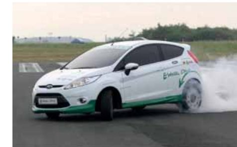
Harmonization of chassis, dynamic handling control, and torque vectoring.
