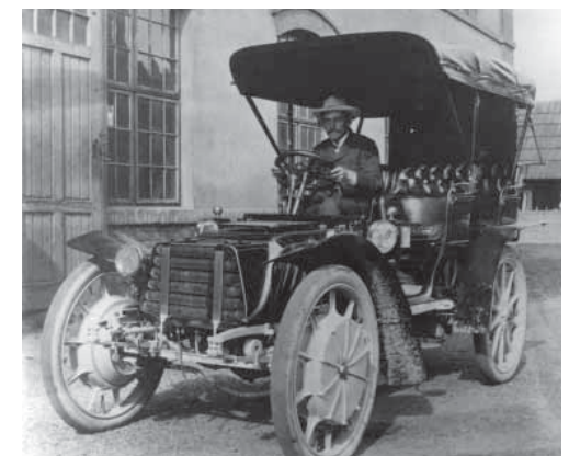
Figure 5 Lohner-Porsche Mixte with gasoline and electric drive (1901) [1]
