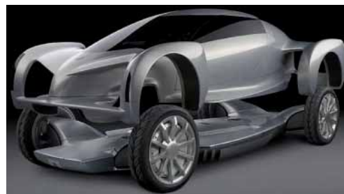
Figure 10 "Skateboard principle" with chassis and body [2]
