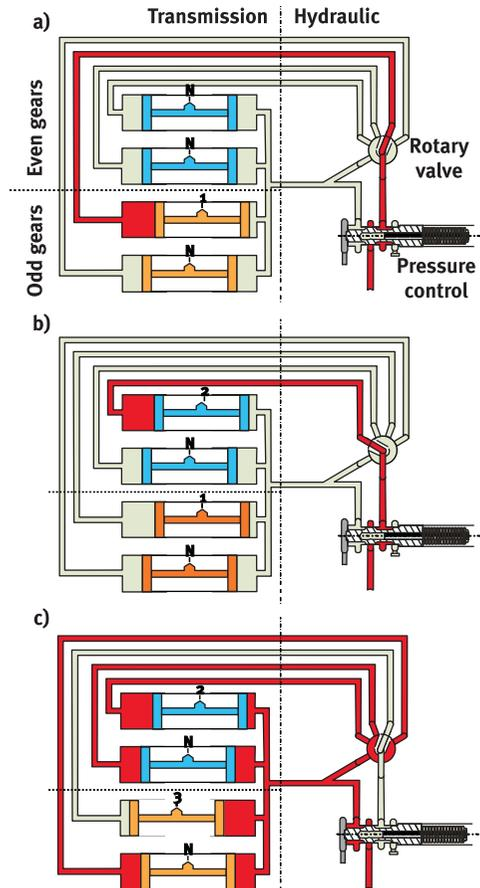
Figure 20 Rotary slide valve for select function
