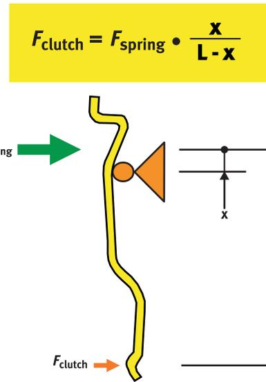
Figure 4 Lever principle
