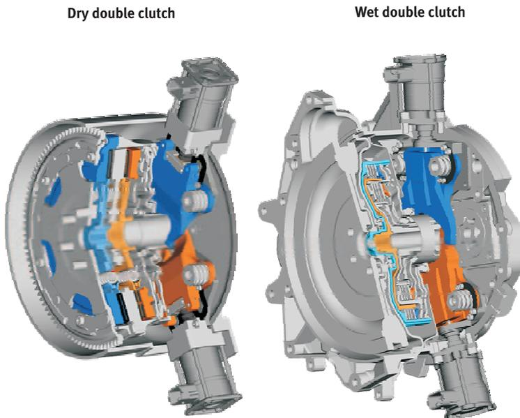
Figure 9 Possible applications of lever actuator
