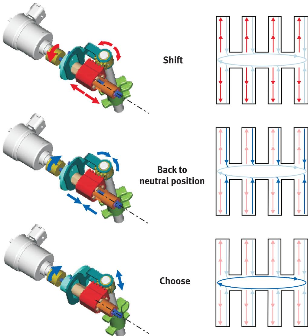
Figure 18 Single motor transmission actuator: function
