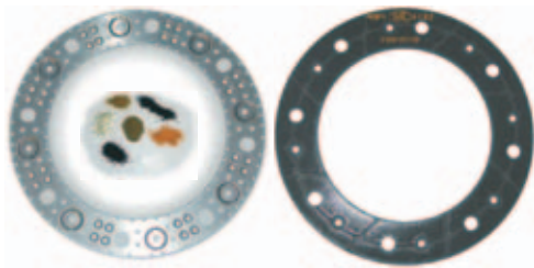
Figure 8 Structure of the LuK RCF-1 facing with steel retainers
