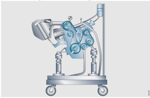
**Test Stand Configuration with Fired Engine**
