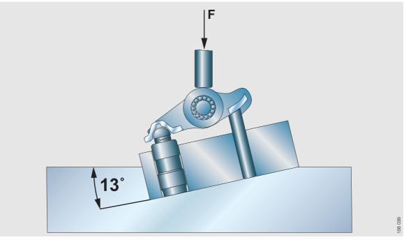
The staircase method is used to test a random sample of 30 parts. If a steel part reaches four million cycles for a particular load level, it is regarded as having withstood the load, and the load is increased one level for the next sample. If a sample is damaged before reaching four million cycles, load is decreased by one level for the next sample.
