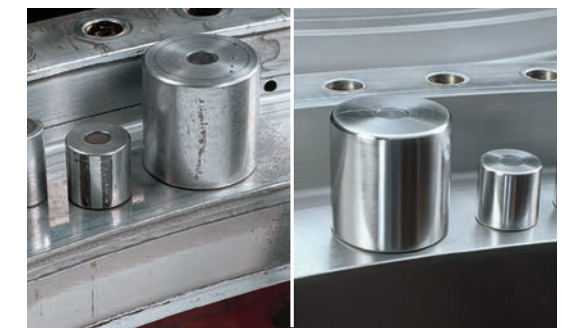
In mint condition: Rolling bearings before and after reconditioning
