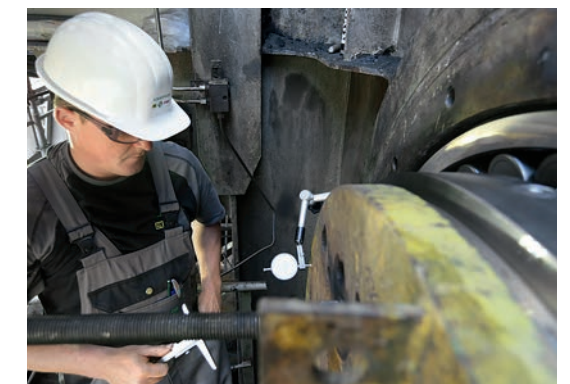
Professional mounting is a must: In statistical terms, 6% of all bearing failures occur due to inappropriate mounting
