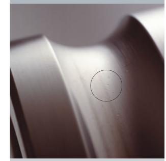
Denting of rolling elements and raceways, causing vibration.
