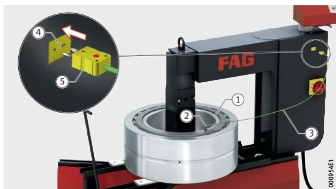
Figure 20 Connecting and attaching the temperature sensor
