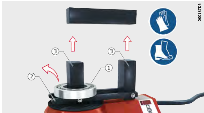
Figure 16 Removing the rolling bearing lying flat
