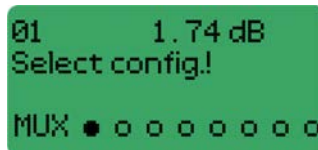
Display to select a configuration
