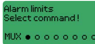
Display showing the sub-menu item to set the pre-alarm limits
