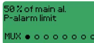
Display to set the pre-alarm limits
