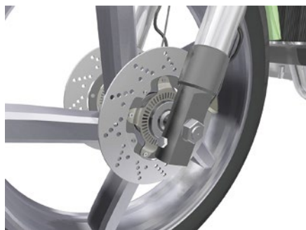
High energy efficiency due to robust wheel bearing with lip seals
