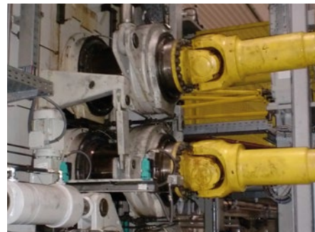
Calender bearing support drive side
