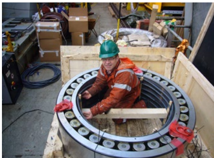
The flexible inductors are wound around the bearing
