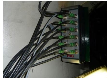
The FAG SmartConnect Box allows the power supply and additional signals to be distributed
