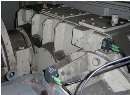
Motor and gearbox monitoring using the FAG SmartCheck
