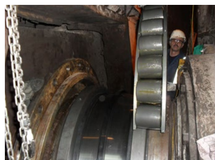
Fitting of FAG split spherical roller bearing
