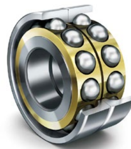
Pairs of angular contact ball bearings in universal design are frequently used as locating bearings in decanters.
