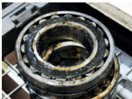
Overgreasing leads to bearing failure
