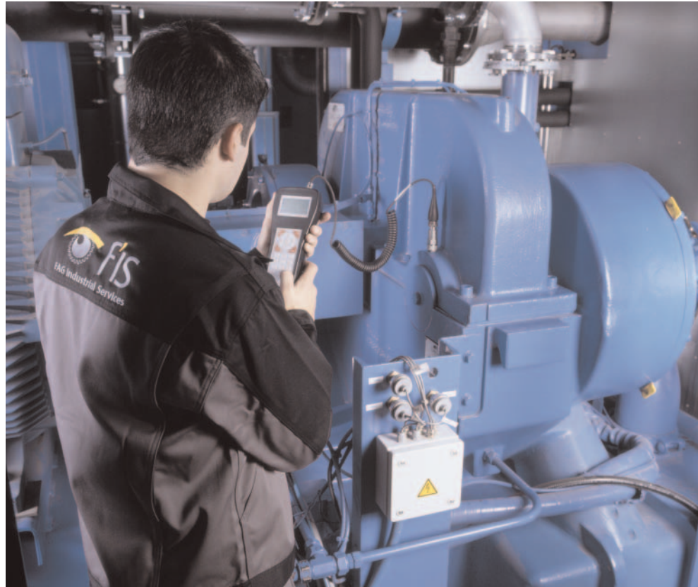
FAG DETECTOR III in use: Monitoring the bearings in an electric motor and in a compressor.
