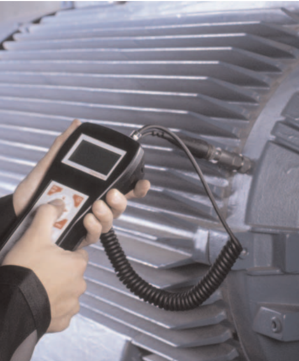
FAG DETECTOR III in use: Monitoring the bearings in an electric motor and in a compressor.
