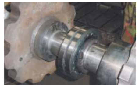
Drive bearing arrangements in conveying and transport equipment
