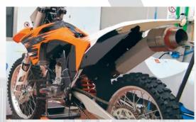
Schaeffler carries out vehicle starting tests in order to inspect the function in the application itself.
