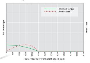
The increasing requirements for reduced fuel consumption and CO<sub>2</sub> emissions mean that friction losses in the engine must also be continuously reduced. This is why the spring forces in the roller one-way clutch are designed to be at a minimum in the idling speed range. When the engine speed increases, the centrifugal force allows the rollers to lift off from the shaft, and the level of friction in the one-way clutch drops to zero.
