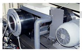
To analyze their operating life, the one-way clutches are tested in the clamping direction using special test rigs. These tests are carried out using the original adjacent parts from the customer's application.
