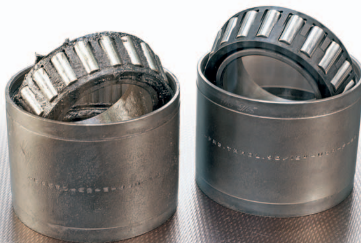
As good as new: Ensuring that reconditioning is carried out professionally and independent of the manufacturer means that axlebox bearings can achieve their maximum operating life.
