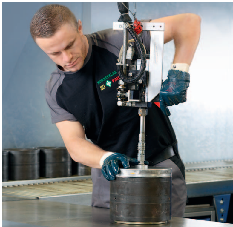
As good as new: Ensuring that reconditioning is carried out professionally and independent of the manufacturer means that axlebox bearings can achieve their maximum operating life.
