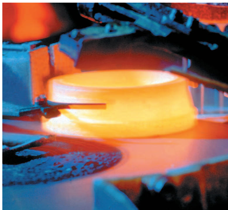
Schaeffler's forging (image above) and subsequent turning processes form the backbone of component manufacture. During the assembly process, the various components are paired together (images below).
