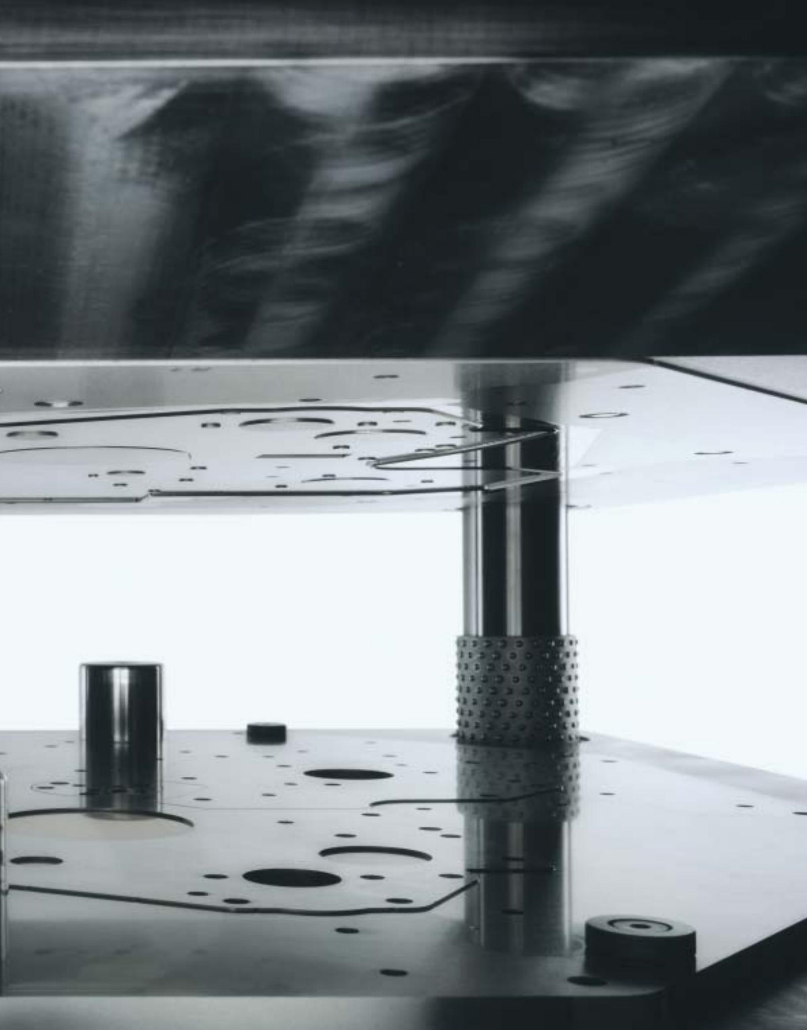
Tool technology is at the heart of fine blanking. In our own tool shop, we use ultramodern methods such as FEM simulation to produce complex tools and dies that combine blanking, drawing, coining and bending processes in one course.
