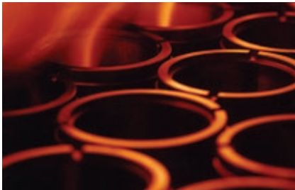
Protection against premature material fatigue: Hardening of inner rings
