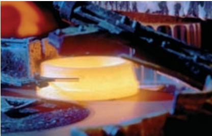
The first step: Forging bearing rings
