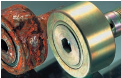
Say good-bye to rust: Corrosion protection with Corroprotect® coating (comparison after salt spray test)
