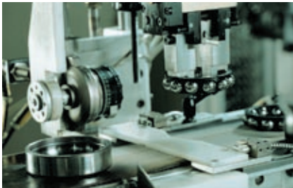
Fully automatic: A complete bearing is manufactured with inner ring, outer ring, balls, cage and grease
