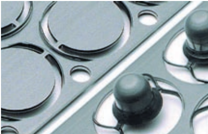
Economically produced: Deep drawn parts at various manufacturing stages
